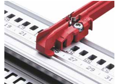
06197001 Sequential numbering on horizontal rails (> 28 HP) and markings on the guide rails provide quick optical positioning aids. ESD clips can be used at front or rear, to protect electronics from electrostatic discharge
