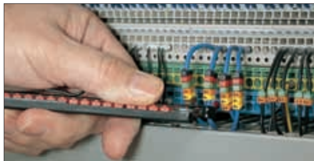
Use the applicator to simply snap the marker onto your cable.
