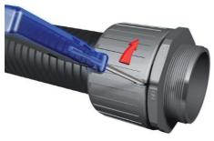
3. Move the handle of the screwdriver towards the "off" position. The capnut will rotate slightly. The locking mechanism is now released.
