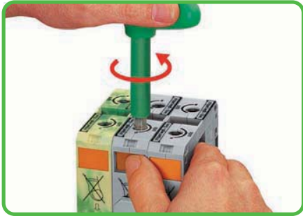
Counter-clockwise rotation using a hex wrench. Orange latch holds clamp open.
