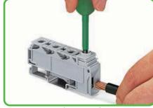
Terminating a 35 mm<sup>2</sup>/AWG 2 conductor. Screw clamp connection, side-entry wiring.
