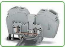
Commoning a 285 Series terminal block (35 mm²/AWG 2) with a 281 Series terminal block (4 mm²/ AWG 12) using a 283-414 step-down jumper. Step-down jumpers are simply pushed down for full insertion, similar to adjacent jumpers.
