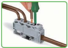
Terminating a 10 mm<sup>2</sup>/AWG 8 conductor CAGE CLAMP® connection, front-entry wiring.
