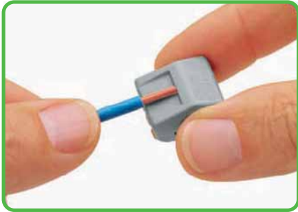
Strip conductor to 9 - 10 mm / 0.37 in.
