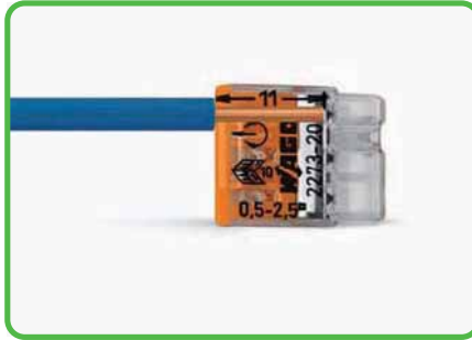
Strip solid conductor to 11 mm / 0.43 in (see marking).
