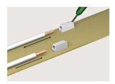
Insert fine-stranded conductors – and remove all conductor types – via operating tool. Connect solid conductors via push-in termination.
