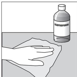
The surface must be dry, free from dust, oil, oxides, parting agents and other impurities. The surface to be glued should be cleaned using a clean cloth and isopropanol / water (50/50). When using other appropriate cleaning agents, ensure that they do not attack the surface or leave any residues.
