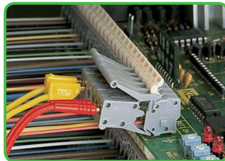
Testing with test plug modules.
